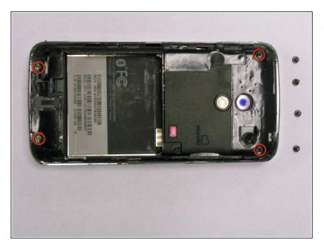
Remove the 4 screws using the T6 screw driver.
