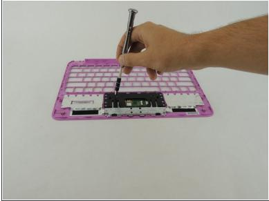
On the back of the plastic keyboard cover, remove the two 2 mm Phillips #000 screws.
