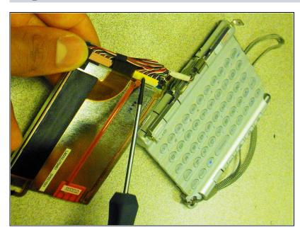
• Quickly release and disconnect the thick cable with your hands.
