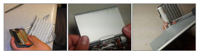
• Gently remove the back plate of the tilt screen by sliding it upward.
