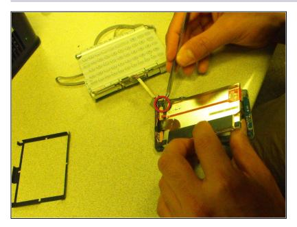
Disconnect the thin connector from the face plate using <u>tweezers</u>.
