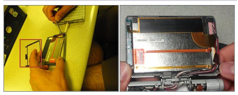
• Detach the plastic black frame from in between the plate and the LCD.
