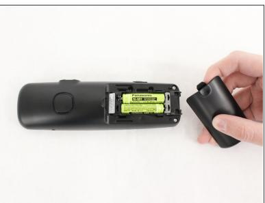
Flip the handset over to expose the back panel, and slide the panel out to remove.
