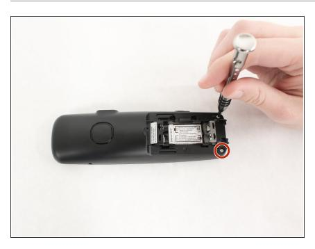
Remove the two screws behind the battery panel by using a Philips size #00 screwdriver.
