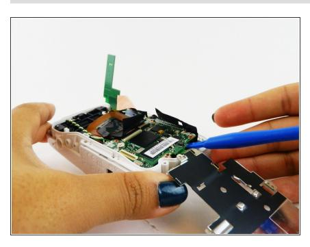
Gently pry off the motherboard using a plastic opening tool.
