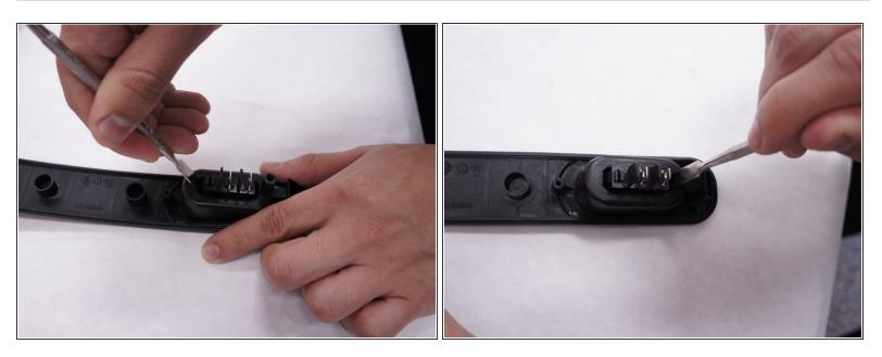
Using the spudger, take out the switch. Do this by pushing the spudger against the switch on both sides as shown and then pull the switch out.
