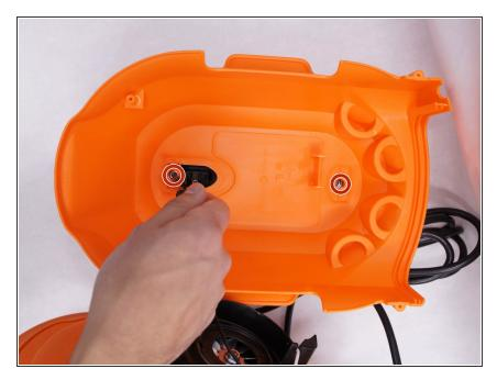
Using a PH2 screw head, unscrew the two 15mm screws as shown.
