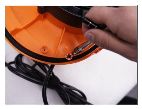
Remove the 15 mm T20 screw. This screw is located nearest the power cord.
