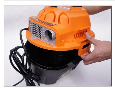
Remove the orange main housing unit from the vacuum bucket by pulling outward on the handle tabs while lifting upward as shown.
