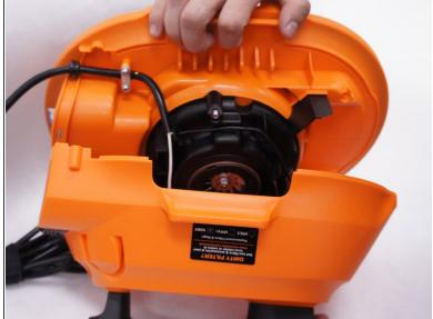
Gently separate the upper and lower sections of the main housing.
