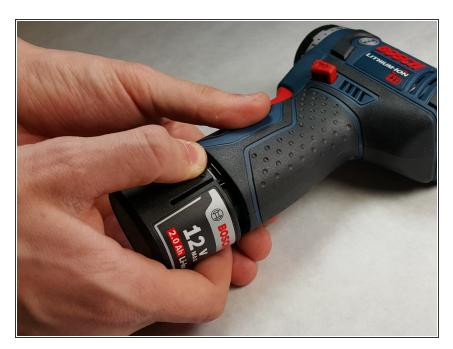
Pinch the two release tabs on the sides of the battery, and slide the battery out.
