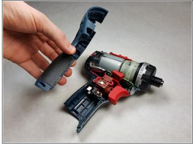
Starting at the rear of the drill, use a wedge to separate the two halves of the outer case at the parting line.
