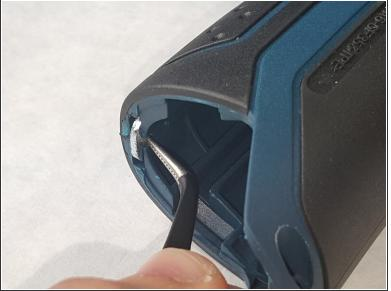
After removing the battery pack, locate the clip that connects the two halves of the outer casing shown in the picture. Remove the clip using angled tweezers or a similar tool. Save the clip for reassembly.
