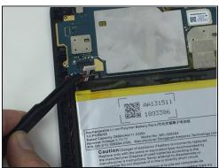
Using angled ESD precision <u>tweezers</u>, lift up on the battery cables to separate the battery connector from its socket.
