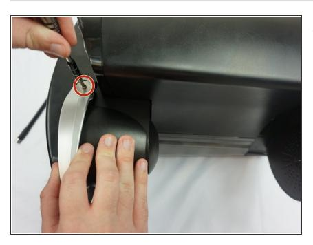
Unscrew one of the 2mm screws on the handle using a T15 screw head.
