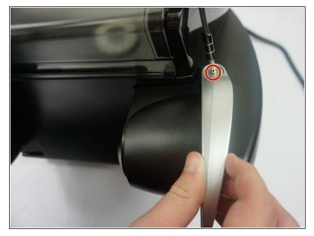
Flip the Keurig over and unscrew the other 2mm screw using the same screw head. Keep a firm grip on the device to prevent it from shifting or falling.
