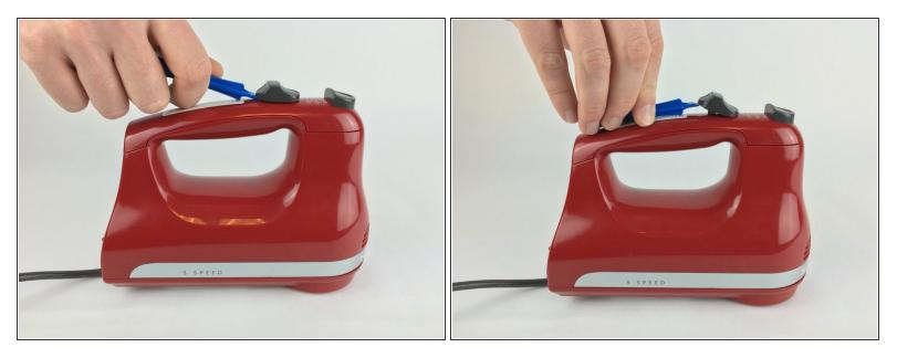
• Use a plastic opening tool to pry off the speed knob.
