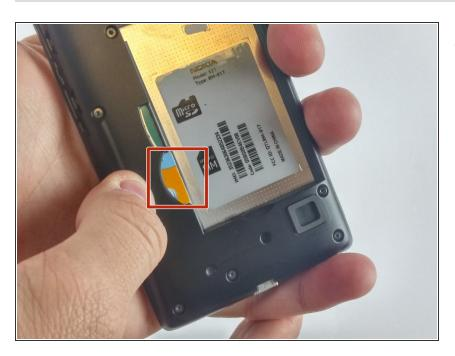
After the battery is removed, push the SIM card from the left side with your thumb until it is loose.
