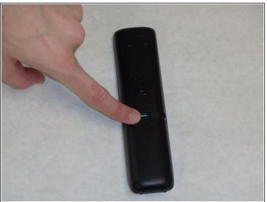
Push down on the battery cover in the direction of the arrow located on the back of the phone.
