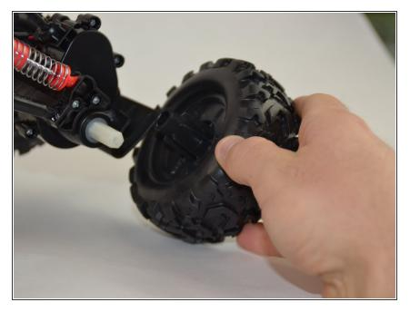
• Remove the tire and determine if the tire is damaged or being obstructed.
