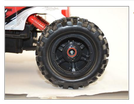
• Use the driver and bit PH2 to remove the 16.1 mm screw.
