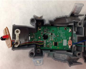
• Use the soldering iron to remove the two wires from the motherboard. Directions on how to solder can be found <a href="here">here</a>.
