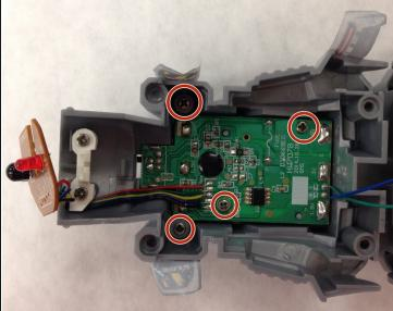
• Remove four 4.75mm screws from the motherboard.
