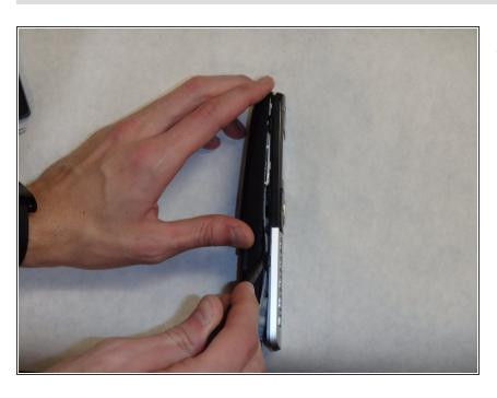
Use the plastic opening tool and spudger to pry the back side of the phone off.
