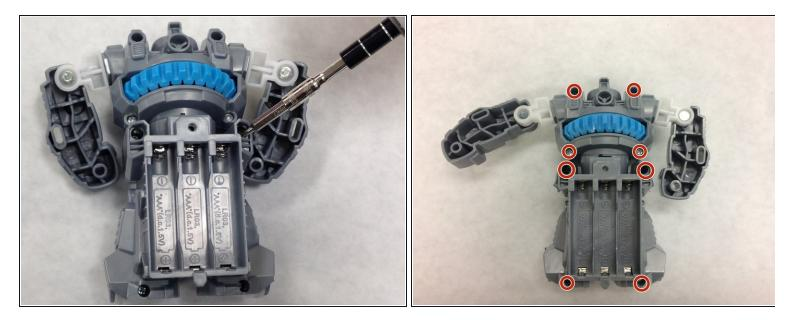
• Using a Phillip #0 screwdriver to remove the eight 8 mm screws.
