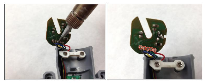
• Use the soldering workstation to remove the five wires. Directions on how to solder can be found <u>here</u>.
