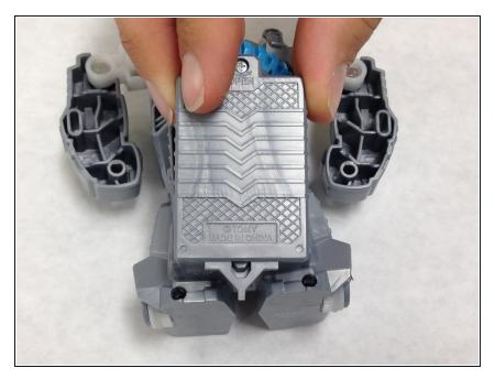
• Lift and slide the batter cover away from the tab holding it in place at the bottom.
