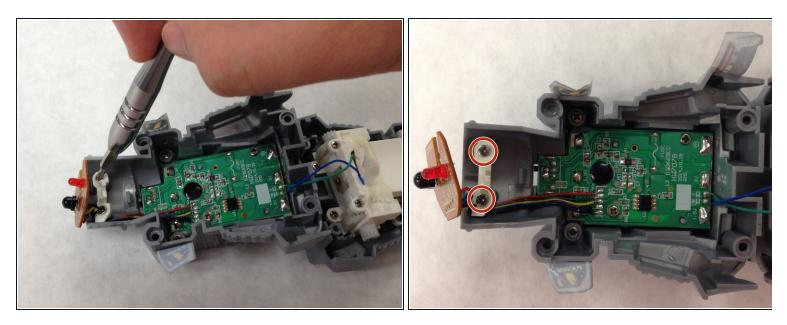
• Use the Phillips 0 screwdriver to remove two 4.75mm screws.
