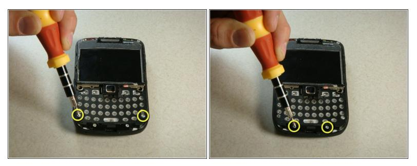
Now there are four screws that need to be removed. They are located at the bottom of the phone and can also be removed using a T6 Torx Screwdriver.
