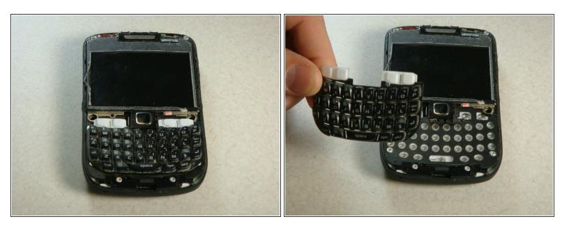
• The keyboard should slide off of the phone now that the plastic siding has been removed.
