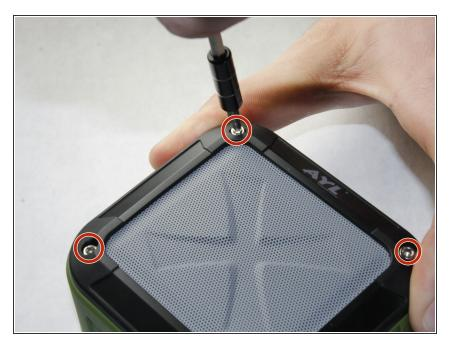
Remove each of the 4 screws on the front cover using the 2.5mm Hex Bit in the screwdriver.
