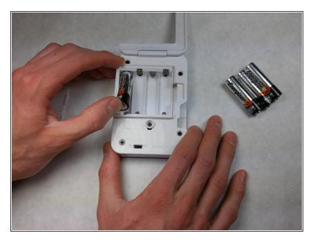
Remove the batteries from the device, allowing you to access the screws necessary for removal of the back panel.
