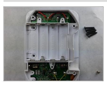
Gently and slowly pull the back cover off of the iGrill, exposing the power cables to the motherboard.
