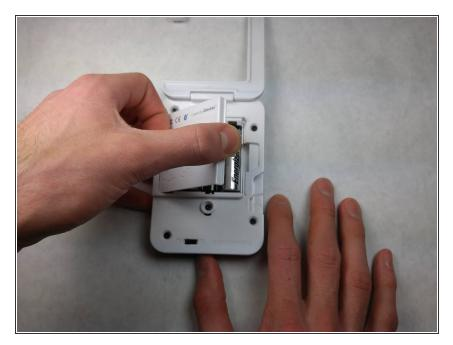
Place the front screen of the device on a flat surface, this allows access to the back cover. Remove the back cover from the device to access the batteries.
