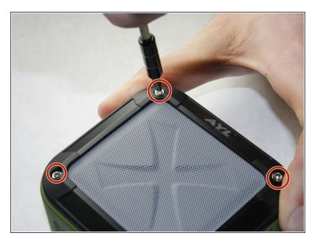
Remove the four hex screws on the top of the device using a 2.5 hex screwdriver.
