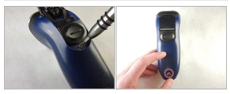
Using a T8 torx screwdriver, remove both 2mm T8 screws.
