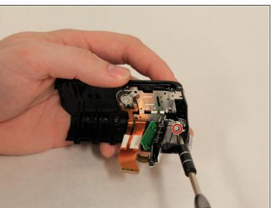
Remove the three 6mm Philips #000 screws holding the black record piece.
