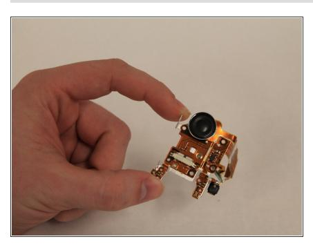
Replace the defective speaker with a functioning one.
