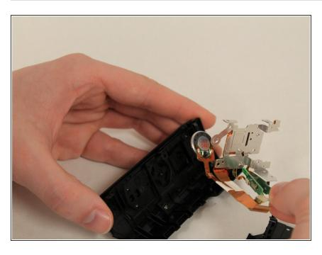
Carefully remove the the whole metal frame out of the device piece.
