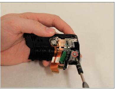
Holding the full top piece remove the six 5mm Philips #000 screws holding the metal frame to the top piece.
