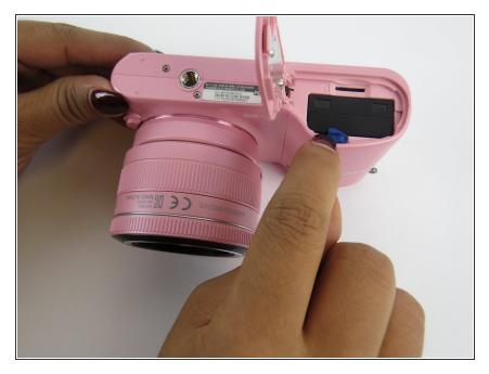
Locate the blue release lever holding the battery down. Slide the blue lever to the right to release the battery itself.
