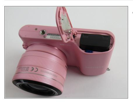
The battery will now slide up about an inch allowing the battery to be pulled out of the camera.
