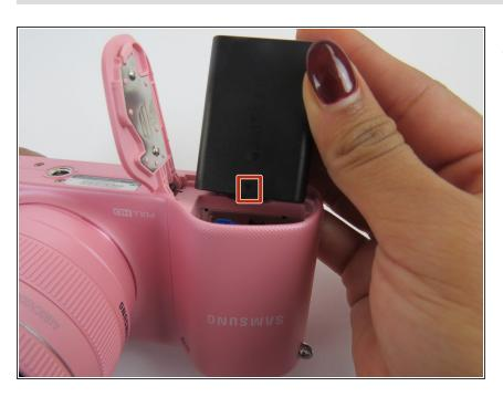
Insert the new battery with the arrow on the battery pointing into the camera. The red square indicates the location of the arrow.
