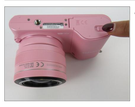
Locate the sliding latch on the right side of the camera and slide the latch to the left side to open up the battery compartment.
