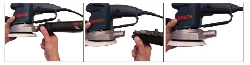
Press the pinch point tabs located on each side of the dust canister and slide the dust canister away from the sander.
