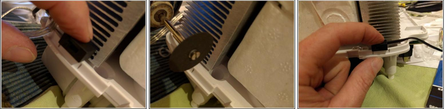
**⚠ Caution.** By cutting this flange (and drilling the holes in the next step), you will be defeating a safety feature of this unit. In the case of internal leaks, or a water spill by the filler neck, water may now **not** be captured by the deck, and would be able to flow down onto the electronics area.
