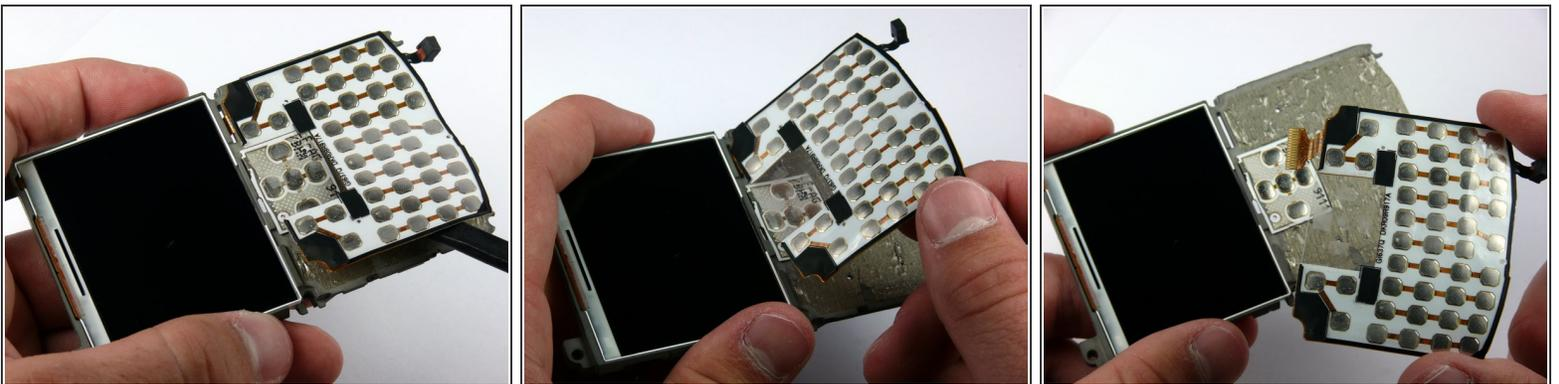
**⚠** The keyboard ribbon cable passes through the LCD frame. Be careful not to rip the ribbon cable when removing the keyboard.
