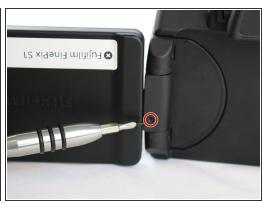
Remove the 4 screws surrounding the LCD screen.
