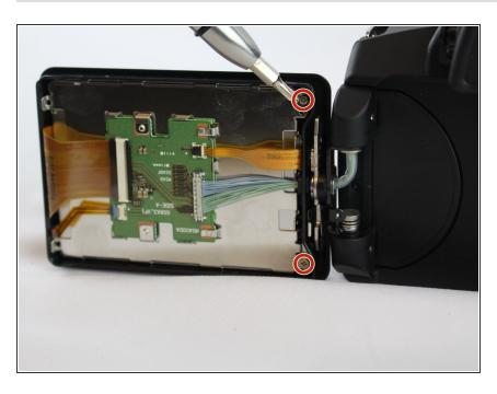
Remove the 2 screws located on the inner corners of the inside of the LCD screen.
