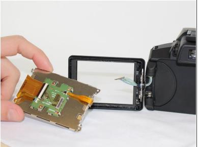
Use a spudger to lift the LCD screen out of its placement and remove it from the casing.
