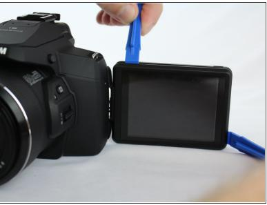
Use an opening tool to pry apart the LCD screen casing and remove the casing.
