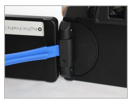
Use an opening tool to remove the casing on the hinge of the LCD screen.
