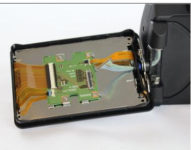
Disconnect the blue cable set by carefully prying it off with a spudger.
