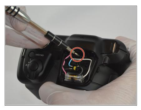
Fold the lid down in order to access and remove the final M3 x 4mm screw using your Philips Head Screwdriver.
