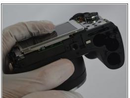
• Once the back plate is removed twist the battery cover clockwise and it should easily dislodge.
