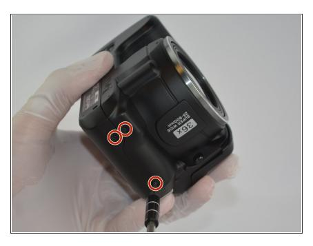
Use your Philips Head Screwdriver to remove the M3 x 4mm screws from the left side of the device as indicated by the pictures.
