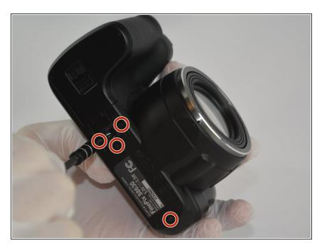
Remove the M3 x 4mm screws from the bottom of your device as indicated by the picture. using the Philips Head J0 Screw Driver Bit.
