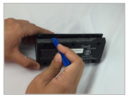
Carefully pull apart the bottom plate and the top plate, using the blue plastic opening tool.
