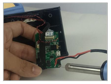
• Desolder the wires that connect the battery to the motherboard, negative (black wire) and positive (red wire).
