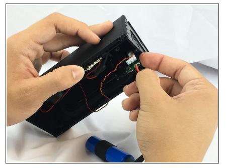
• With some force, push the motherboard straight in toward the center of the device.
