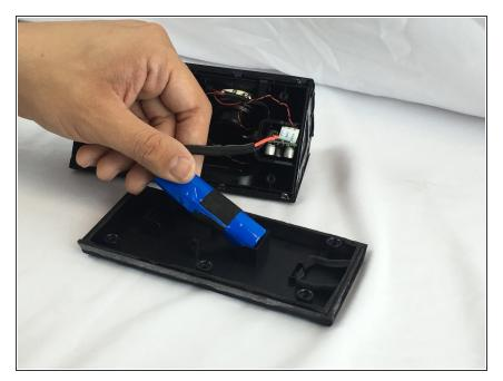
• Separate the battery from the bottom plate and set the bottom plate aside.
