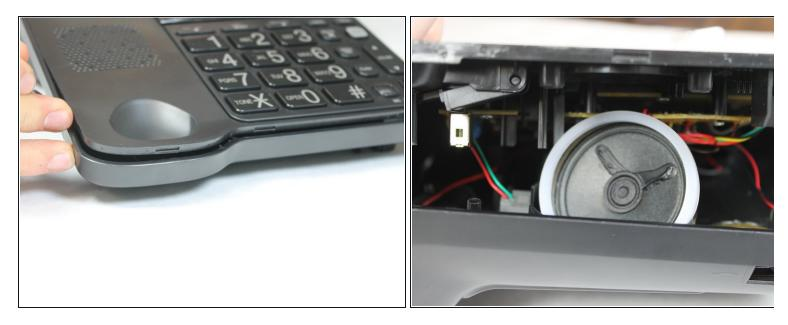
• Remove the front panel of the device as shown.
