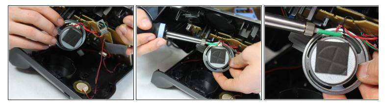
• Desolder the speakerphone with a soldering iron.
