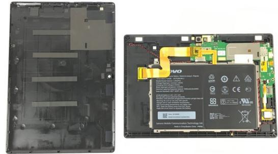
✦ Before removing the battery, make sure the device is powered off
