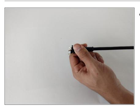
Pull out the cord sleve for the new cable replacement.
