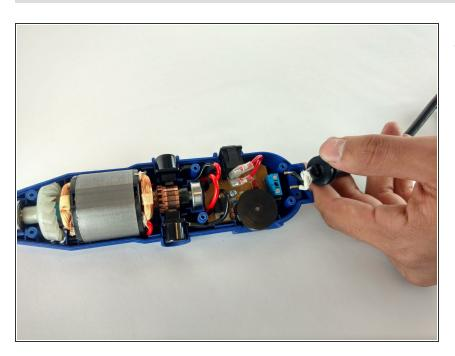
Pull out the power cable connectors.
