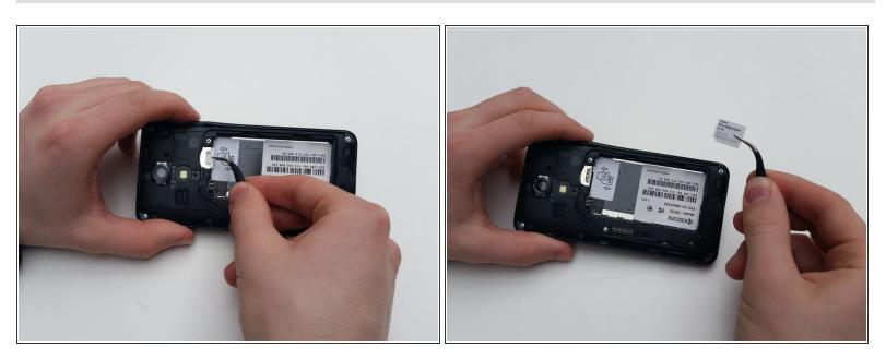
• Use the precision tweezer set to safely remove the SIM card.
