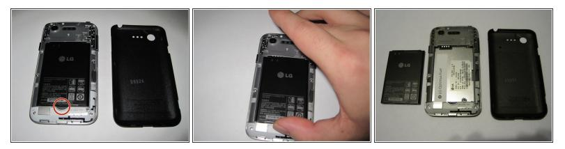
• Use the curved opening at the center-bottom of the battery to carefully remove the old battery.
