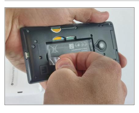
Once the cover has been removed, the battery will be visible. Grab the plastic tab and pull it to remove the battery from its place. If there is no plastic tab, use the plastic opening tool to pry the battery loose. To reassemble your device, follow these instructions in reverse order.
