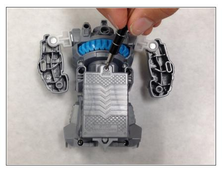
• Using the Phillips #0 screwdriver to remove the 8 mm screw.
