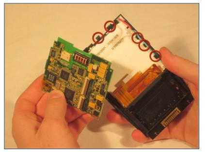
Gently pull the black clips on the inside case to detach the motherboard from the device.
