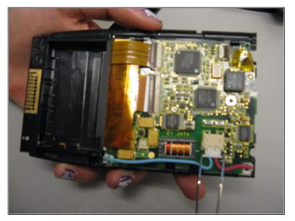
Using tweezers unhook the blue and red screen cables where they connect to the motherboard.
