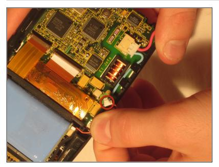
Unhook the battery cable from the motherboard and remove the battery.
