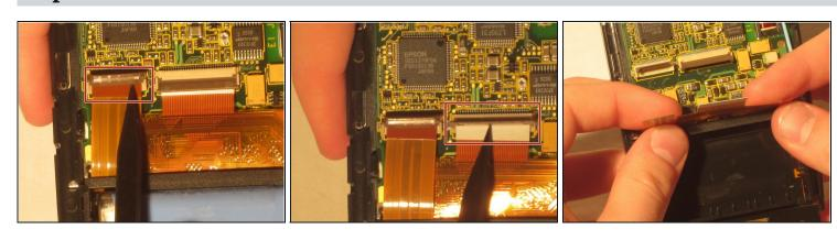
Using tweezers, pull up the other two ZIF connector tabs.
