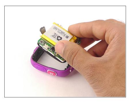
Lift the circuit board carefully from the casing, without breaking or detaching the speaker wires at the bottom of the circuit board.
