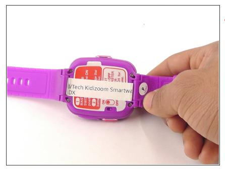
Make sure the master switch is "OFF" before disassembly, to avoid an electric shock.
