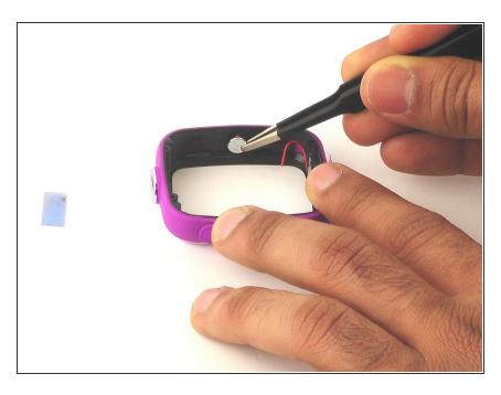
Use tweezers to separate the backside tab from the front side of the button.
