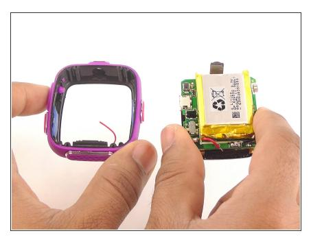
Wait for the solder to cool down and solidify, then remove the circuit board from the casing.
