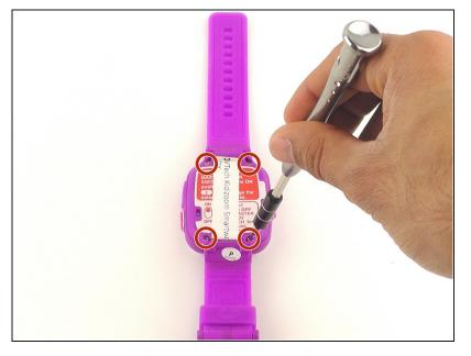
• Remove the four 6.0 mm screws on the back plate with the Phillips #00 screwdriver.
