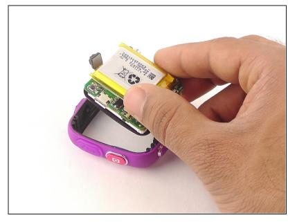
• Lift the circuit board carefully from the casing, without breaking or detaching the speaker wires at the bottom of the circuit board.
