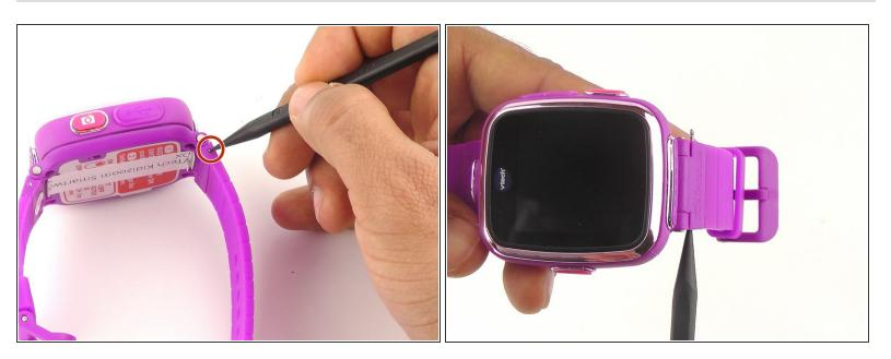
• Use the pointed end of the spudger to push the small-headed pin through the other side.
