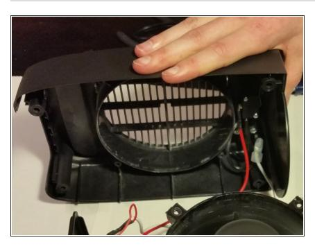
Set the case back on its side, so the safety switch is no longer pressed, and the motor turns off.
