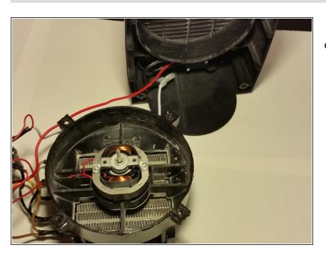
Stand the heater case up, so the safety switch is pressed, and the motor is on.
