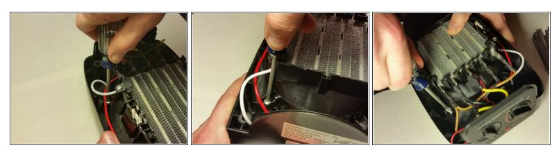
Remove the four Phillips mounting screws from the heater assembly.
