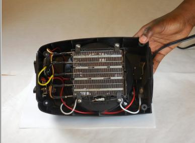
Carefully remove the front heater panel.
