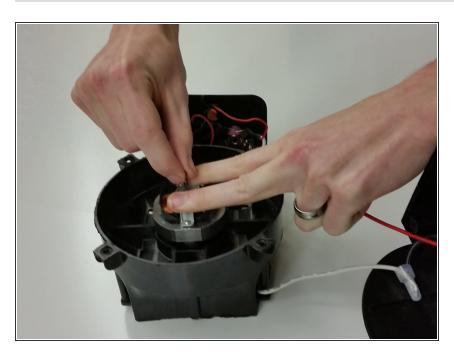
Push down on the motor bracket and adjust the motor by hand so it spins freely and does not scrape.
