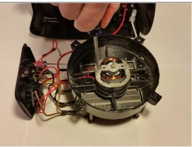
Slightly loosen both of the motor retainer screws about one full rotation.
