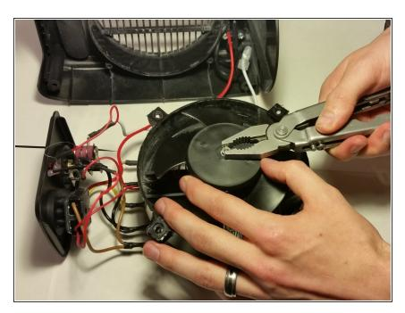
Using pliers, remove the fan's center mounting nut.
