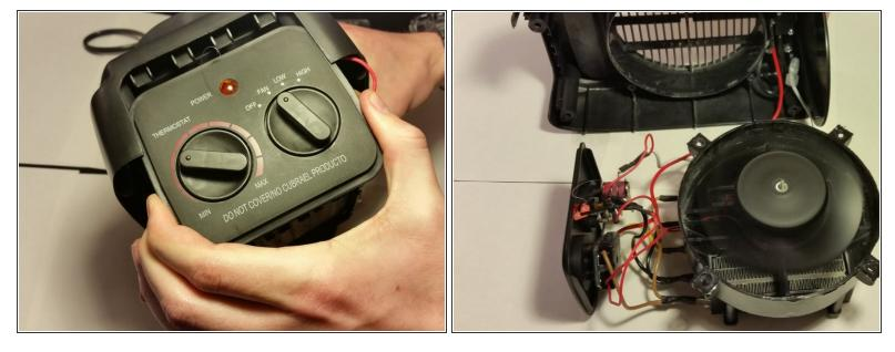
Slide the top control switch panel out. Be careful not to pull, or apply excess pressure to, any of the wires.
