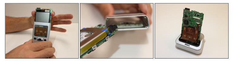
• Slide the motherboard out of the protective case.
