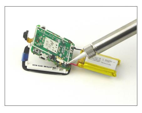
De-solder the red battery wire from the circuit board.
