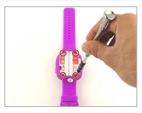
Remove the four 6.0 mm screws on the back plate with the Phillips #00 screwdriver.
