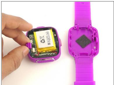
Lift the master switch from the circuit board.
