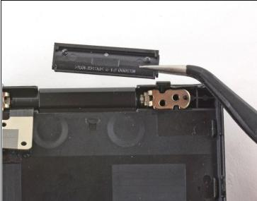
• Use tweezers to remove the plastic cover on the LCD hinge.
