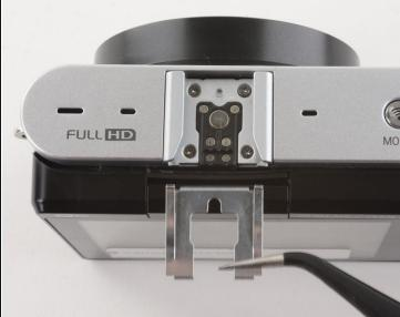
• Use tweezers to remove the metal shield from the external flash mount.
