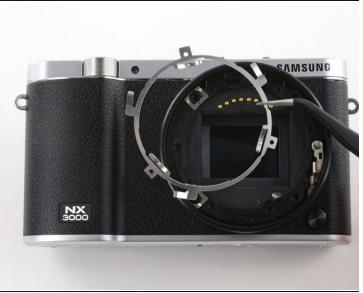
• Use tweezers to remove the black plastic ring and small metal ring inside the lens assembly.
