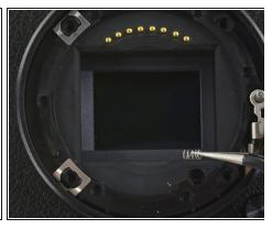
• Use tweezers to lift the pyramid screw and spring from the lens assembly.
