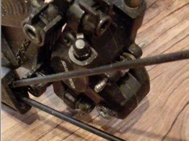
• Loosen the clamping screw with 4mm Allen key / Allen and remove the front wheel from the fork.
