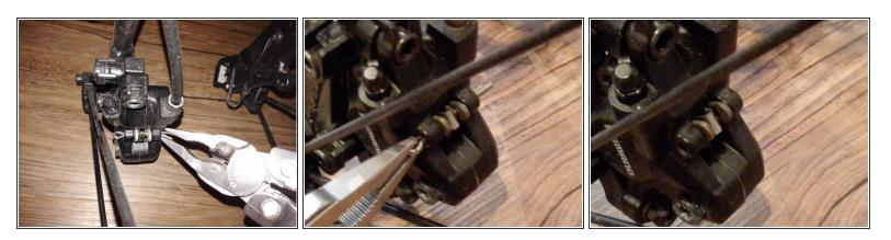
Press the cotter pin together with the pointed pliers at the ends and pull out.
