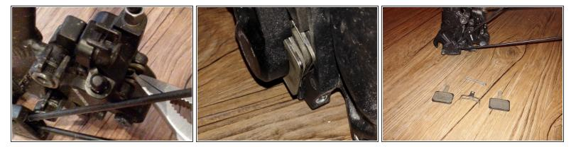
Push the squeaky brake pads out with the needle nose pliers. (For heavily worn brake pads, push the brake pistons outwards).
