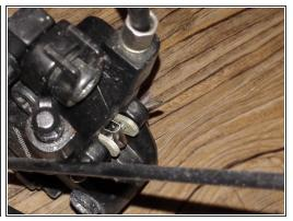
Insert the new split pin and gently press the ends apart with the needle nose pliers.
