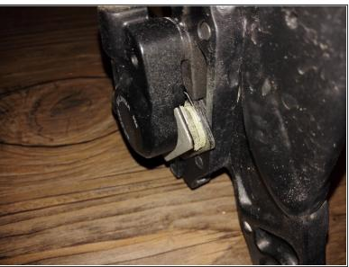
Insert the new brake pads together with the spring into the caliper.
