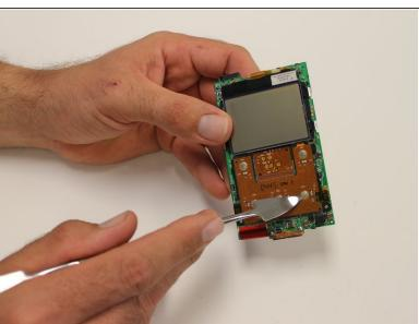
Disconnect side clips of screen to detach the base of it from the main circuit board, using the metal spudger.
