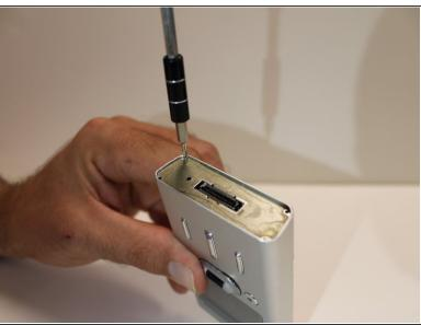
• First, disassemble the device, taking off the bottom panel. See the <u>disassembly</u> guide for further directions.
