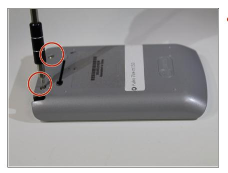
Take the screwdriver from the IFixit toolkit and use the T6 bit. Unscrew the the top two 3mm screws above where the flap was connected to the device.
