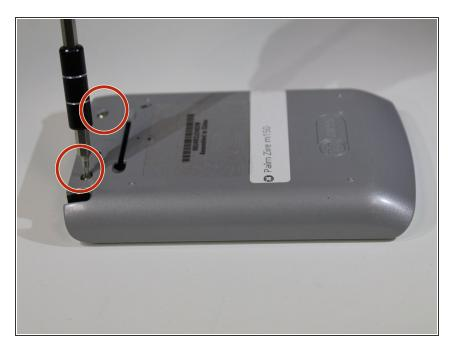
Take the screwdriver from the IFixit toolkit and use the T6 bit. Unscrew the the top two 3mm screws above where the flap was connected to the device.
